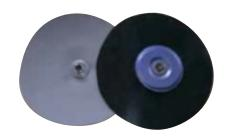
Main component of the RUBBERFIX SYSTEM  $^{\circledcirc}$  features a threaded insert  $\emptyset$  10 mm on the upper part (disk in  $\emptyset$  20 cm in SINTOFOIL or SINTOPLAN) and a black washer on the lower part treated for induction welding, on which the threaded insert is fixed.
