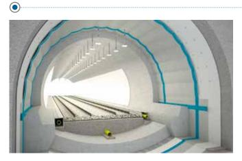
This system integrates the previous system with the compartimentation of the surfaces with special PVC-P or TPO joints thermal fusion welded to the sealing element.
