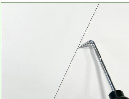
6. Testing. Check the welds with the appropriate hook tool..
