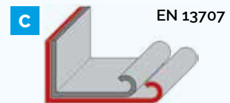
Multi-ply exposed systems Lower ply
